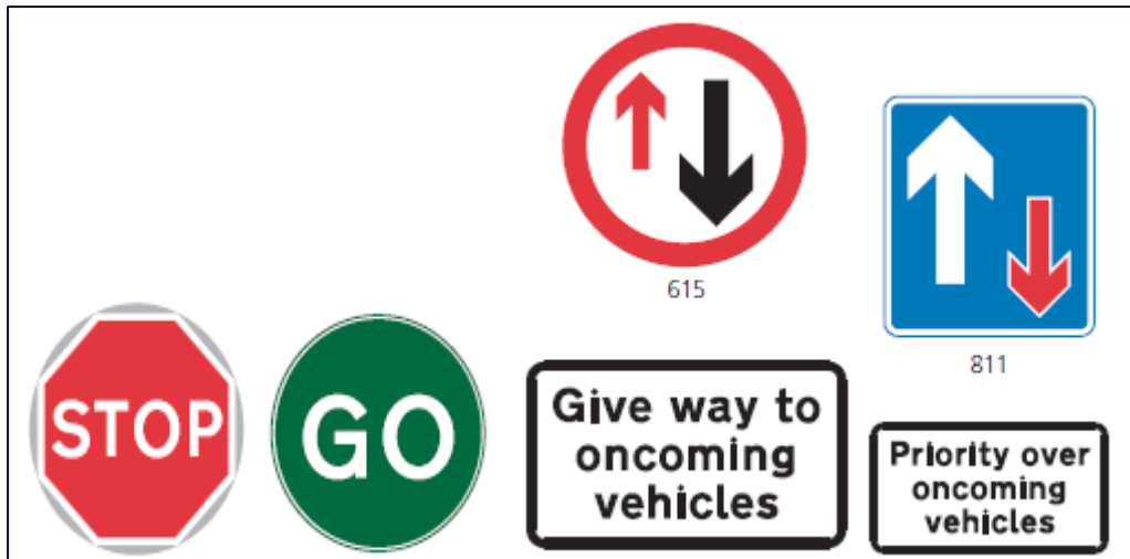
Figure 1.5: Manually operated stop/go signs and priority signs.
